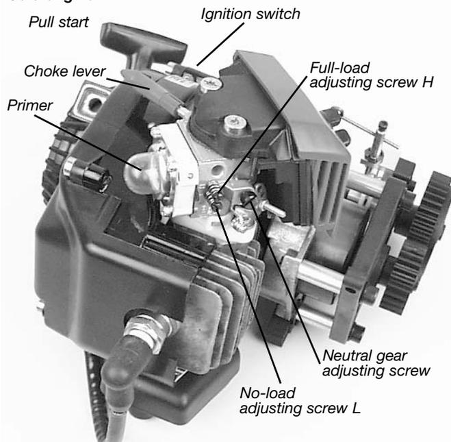
During the first two tank fillings you should avoid maximum speed ranges in no-load condition as well as longer full-speed drives on parking places. The first thing we recommend to check is the effective radius of your radio control system with running engine.
